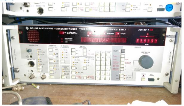
9kHz to 30MHz Test Receiver.
