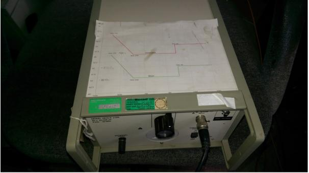
This is used to safely and accurately measure the amount of interference injected into the mains supply by the device under test.
